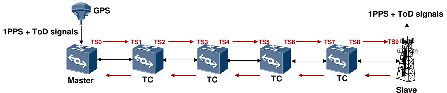
$$\text{Route delay (Master to Slave)} = \text{TS9} - \text{TS0} - (\text{TS2} - \text{TS1}) - (\text{TS4} - \text{TS3}) - (\text{TS6} - \text{TS5}) - (\text{TS8} - \text{TS7})$$
